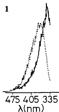
Figure 5. Fluorescence spectra of jet-cooled 1 excitation at 324.41 nm (●—●) and 323.29 nm (●⋯●), corresponding to excess energies of 60 and 166 \text{cm}^{-1} , respectively.
